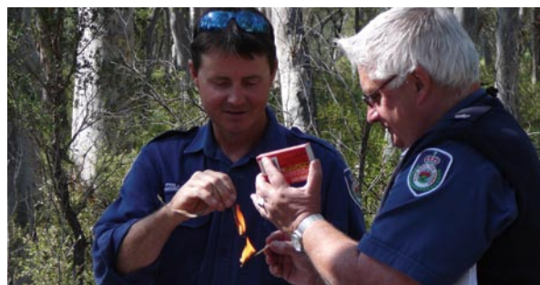
Phil Worner and David Stimson demonstrate the 'leaf test'. This helps determine how much moisture there is in vegetation.
